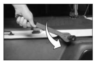
Turn the ratchet counterclockwise to lower the spare tire to the ground. If the spare tire does not lower to the ground, the secondary latch is engaged causing the tire not to lower. See Secondary Latch System on page 5-79.
